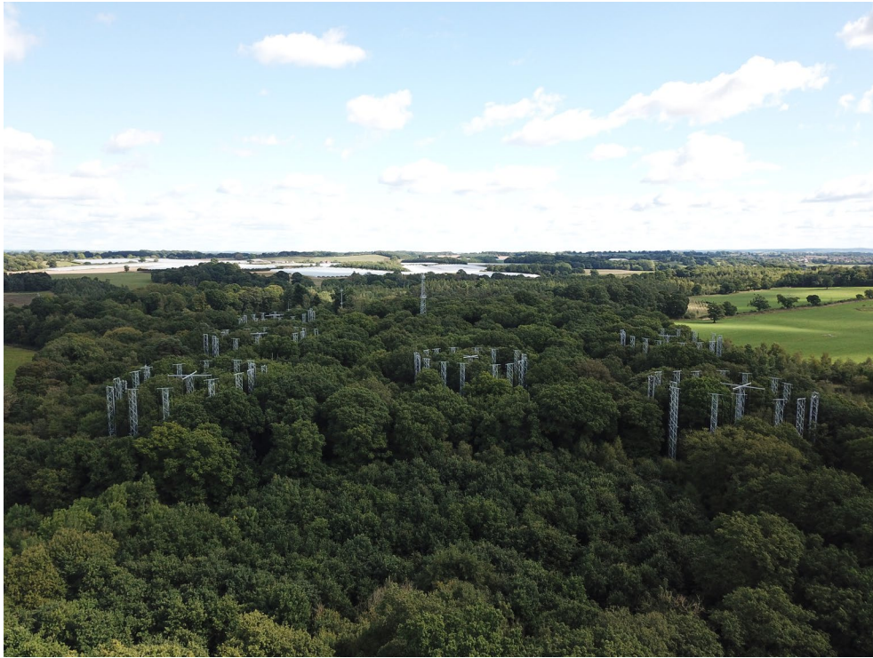
Extended Data Fig. 1 | Aerial view of the BIFoR FACE facility. The research site comprises six experimental arrays of c. 30 m diameter and a flux tower. Photo by Peter Miles, University of Birmingham.
